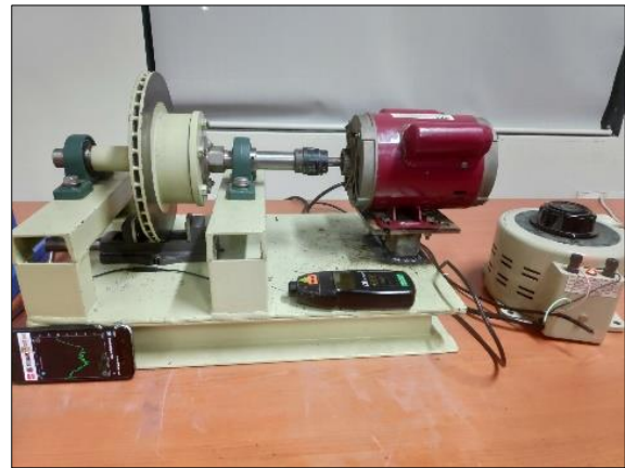
Figure 5: Experimental Setup for squeal measurement
